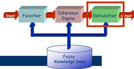
Converts the **fuzzy output** of the inference engine to **crisp** using membership functions analogous to the ones used by the fuzzifier.
